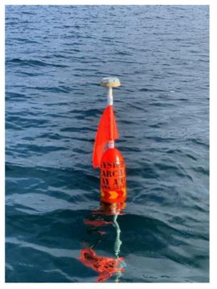
placed on the lake bottom in waters generally more than 90 feet to pick up signals from the acoustic tags as cisco swim by. These receivers are anchored to the bottom of the lake. Interfering with the acoustic equipment will jeopardize research results.
